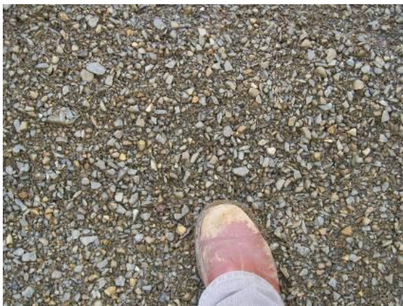
Figure 14 Granular fill material [4]
