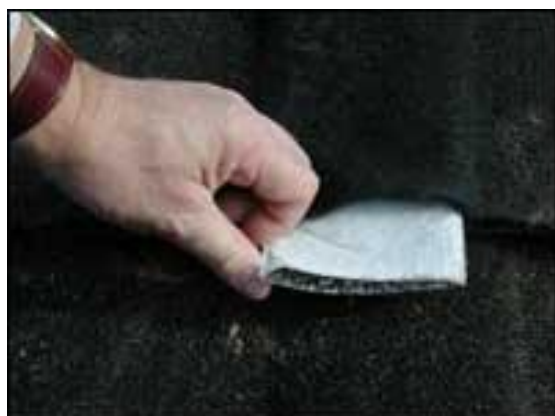
Figure 32 PVD geocomposites provide effective ground improvement solutions [8] & [4]
