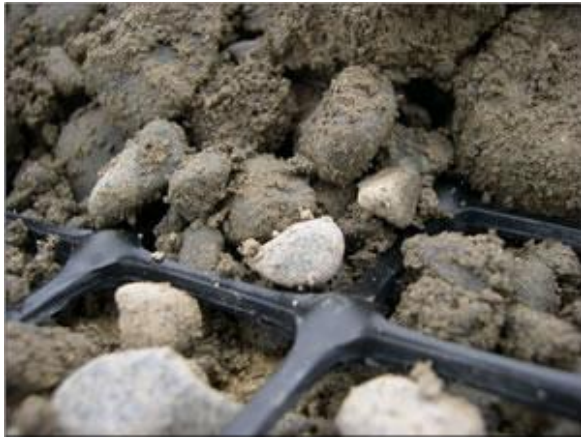
Figure 36 The reinforcement of unpaved roads often utilises bi-axial geogrids [19]
