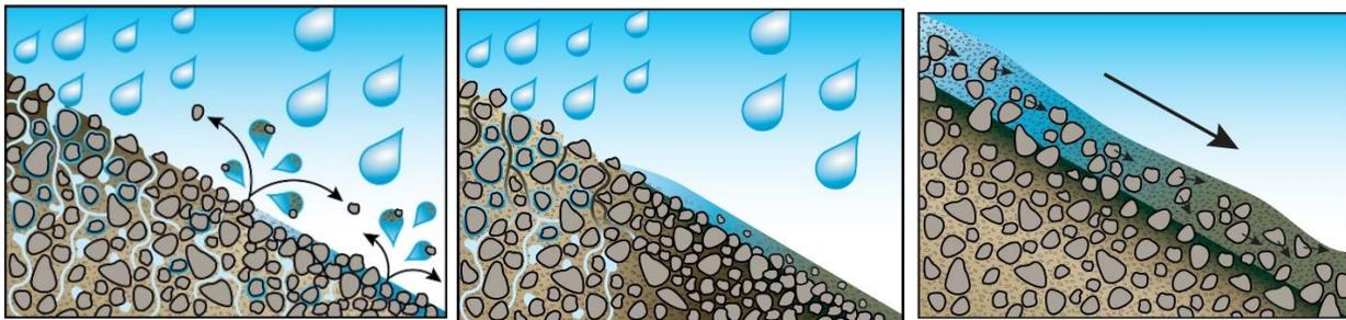
Figure 2: a. Erosive precipitation hits a slope surface b. Pore blockage c. Surface runoff with material transport
